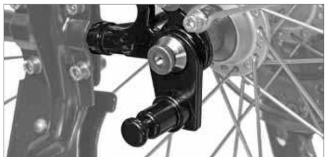
the tension-adjusting nut adequately may result in accidents with serious injury or death. If the quick-release skewer is too short, it must be replaced. Consult a professional bicycle mechanic for the appropriate parts and assistance.
